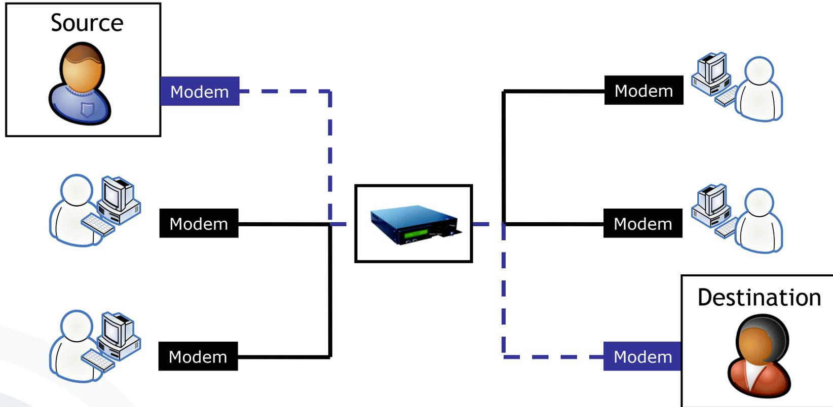
In circuit-switched networks, the communication line is used exclusively for the communicating parties (similar to the phone system, CSD and HSCSD).
